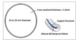
**Figure 1:** Bimatoprost ocular insert. Schematic representation. An inner polypropylene structural ring covered with a siliconebimatoprost matrix for slow release of bimatoprosrt. Figure is adapted with permission from "Brandt JD, DuBiner HB, Benza R, Sall KN, Walker GA, Semba CP, *et al.* Long-term Safety and Efficacy of a Sustained-Release Bimatoprost Ocular Ring. Ophthalmology. 2017;124(10):1565–6"
