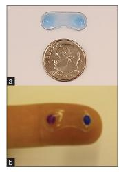
**Figure 3:** Topical ocular drug delivery device. (a) The clear elastic matrix of the device. (b) The purple and blue circles mark the drug depot cavities. Curtesy of Amorphex Therapeutics LLC
